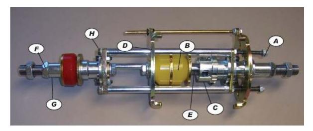
The 3-stage torque link uses a combination of a wire spring and poly spring bushings to absorb engine torque and increase traction to the rear tires. As engine torque is applied the wire spring will compress and the poly spring bushings will engage. As the spring bushings engage the spring rate will increase. This torque link is very tunable. Understanding the various adjustments that can be made is crucial to torque link performance.
