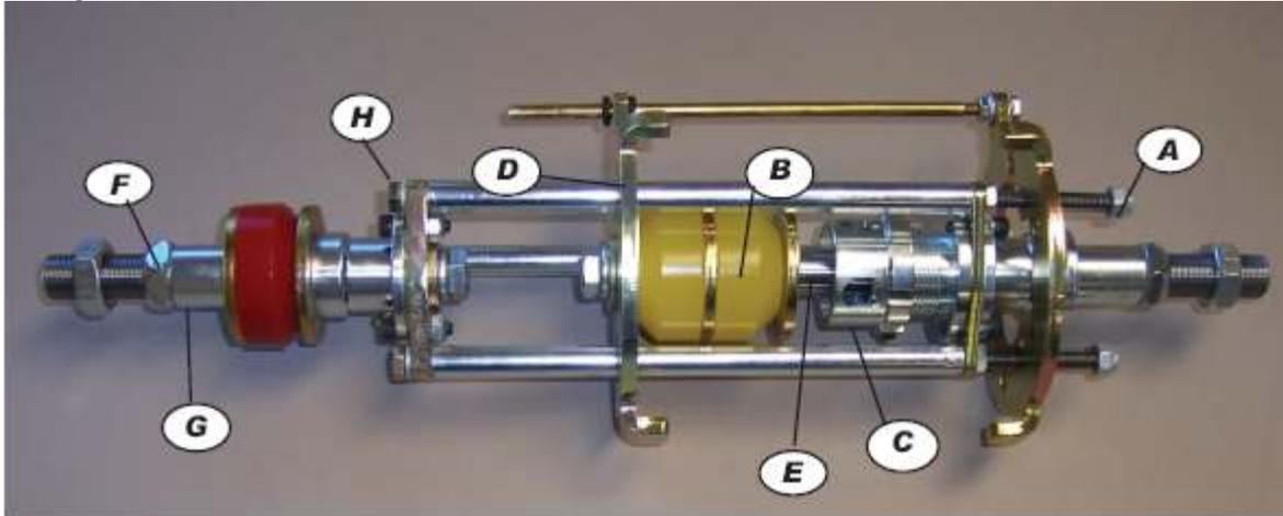
The 3 stage torque link uses a combination of a wire spring and poly spring bushings to absorb engine torque and increase traction to the rear tires. As engine torque is applied the wire spring will compress and the poly spring bushings will engage. As the spring bushings engage the spring rate will increase. This torque link is very tunable. Understanding the various adjustments which can be made is crucial to torque link performance.
